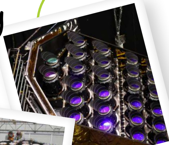
A close-up of PLATO's 26 ultrasensitive cameras.
